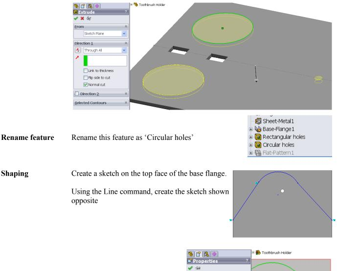
Select the line segment and arc by holding down the 'CTRL' key and apply a 'Tangent' relation
